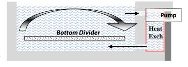
slot at one end. This flow mixes with the heat exchanger discharge. As it emerges from under the bottom divider, the liquid is so close to the mean tank temperature, that gradients are less than 0.002°C throughout the bath.
